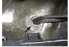
Plug the door sensor into the wiring harness and route it up the door frame, under the carpet.
