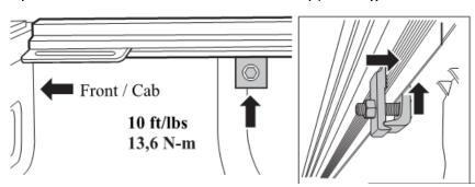
**NOTE:** When installing the rail clamps make sure the clamp is inserted all the way up into the rail, and the clamp teeth are aligned to the rail slots to ensure a secure grip.
