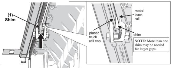
2. Starting with the front clamp, make sure the rail is pushed forward against the bulkhead and square with the bed rail. Apply downward pressure on the rail, insert the clamp as high as possible, ensuring the front bracket is captured, and tighten to 10 ft/lbs.
