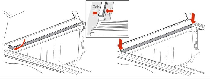
Install foam block bulkhead seals. Clean the top of the bulkhead underneath the bed rail cap. Peel the paper backing from the block and apply to the top of the bulkhead underneath the bed rail cap. Install one block on each side
