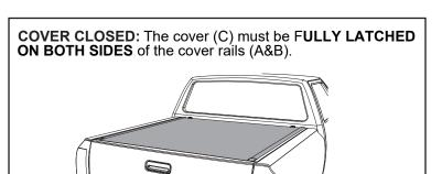
Prior to vehicle operation, the truck bed cover MUST be properly secured.
