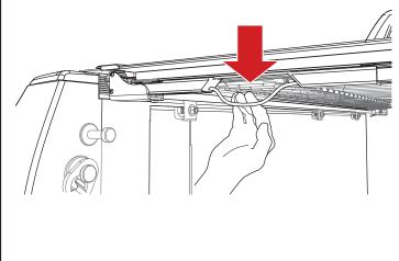
**ROLLED UP POSITION:** To drive with the cover (C) in the open position, use the cover straps (M). Roll the cover forward, twist and insert the clips into the cover clasps. Ensure that **BOTH** strap clamps are fully inserted into the clasps. Pull on the end of the strap to tighten.
