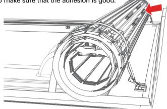
**25** Install one end cap (C) on the rearward portion **ONLY** of the new passenger side cover rail (A), as shown. Tighten the set screw with the provided Allen wrench. Do this also on the new driver side cover rail (B).
