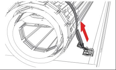
**OPENING COVER:** Pull down on the latch release cable located on either side of the cover (E) and rotate the tail rail forward and into a rolling motion. When driving with the cover open, the cover must be rolled toward the cab and secured with **BOTH** strap clamps.
