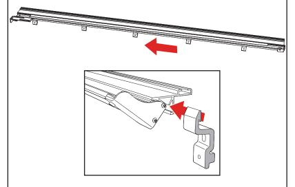
Mount the passenger side rail (A) into the holes in the truck bed. **Reuse the screws from step 6**, using a drill/socket wrench. Before tightening, make the necessary adjustments for the rail so that it has proper clearance to both the front cargo rail and the tailgate. Make sure the passenger side rail is pushed tight up against the front cargo rail.
