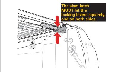
Check to see that the latches on both sides at the tailgate fully engage the cover rails (A & B). Loosening the lock knobs (I) and making the side to side adjustment as in step 19 could help with the latch striker engagement.
