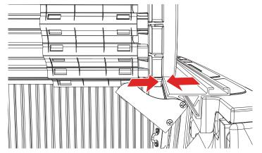
When correctly installed, the vinyl edges of the rolled cover (E) will align squarely with the side rails in all four corners. The latch assembly will align with the side rail locking levers at the tailgate on both sides.
