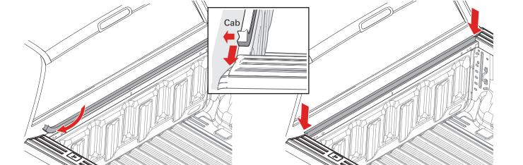
Align the S clamps (G) with the passenger side rail slot and insert into the new passenger side cover rail (A). The S clamps should match the truck bed hole locations.
