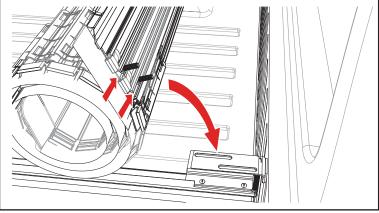
Open and close the rolled cover (E) several times to verify that it rolls freely. The cover should be square with the cover rails and roll freely between the rails.
