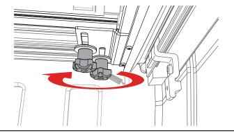
With the cover (E) in the open position, the other end of the strap clamp assembly (F) inserts into the cover clasp and turns to lock. Pull up on the strap end to tighten. Always hook the straps on BOTH sides.
