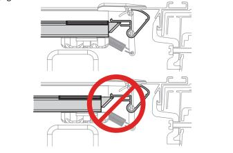
When the rolled cover (E) is properly aligned, roll it open, ensuring not to misalign while opening. Tighten the knobs (I) on both sides to secure the cover. **DO NOT overtighten**. Hand tighten only. Recheck that the cover operates correctly. Close the cover and check that the locking levers are engaged and prevent the hard rolled cover from being lifted on both sides.
