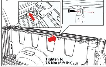
**12 IF YOU DO NOT HAVE A CARGO RAIL**, disassemble the strap clamp assembly (F) and use only the strap, washer and lock washer. Using a screw (H), secure the strap, washer, and lock washer to the first S clamp near the cab end.
