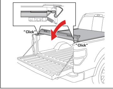
**ROLLED UP POSITION:** To drive with the cover (E) in the open position, use the strap clamps. Roll the cover forward, twist and insert the clips into the cover clasps. Ensure that BOTH strap clamps are fully inserted into the clasps. Pull on the end of the strap to tighten.
