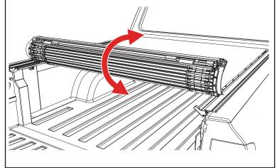
Verify that a gap of approximately 1/8" (3.2mm) remains on both sides of the rolled cover (E) between the edge of the cover rail and the rolling cover. This spacing is necessary to ensure that the locking rail secures to cover. Align the cover side to side at the front and/or the back if the side gaps are not even. Firmly hand tighten the knobs (I) after the cover has been aligned.
