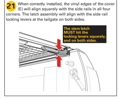
Check to see that the latches on both sides at the tailgate fully engage the cover rails (A & B).
