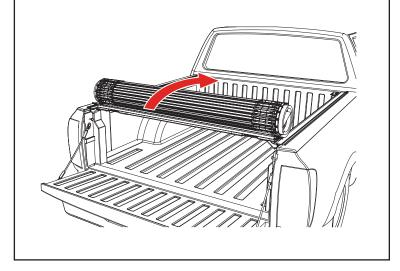
Fold the front panel back and insert the two mounting bolts (M) into the slotted bracket. Do this for both sides The bolts will align with the slotted bracket of the cover rail. Fold the panel back down.
