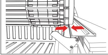
With the cover (C) closed, push the cover toward the tailgate to position it for contact with the D-seal and the tailgate.
