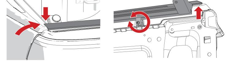
Rest the rolled cover (E) onto the rails at the tailgate, roll the cover toward the cab, and remove and discard all packaging materials.
