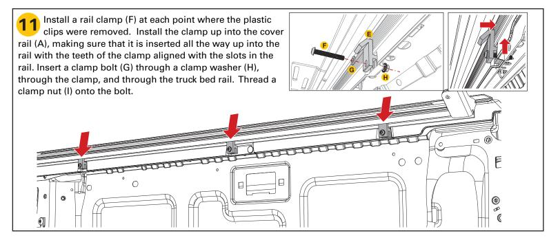
Starting with the front clamp (F), apply downward pressure to the cover rail (A & B) while tightening the bolt. Tighten to 8 ft/lbs (11 Nm) of torque. Repeat with the middle and then rear clamp, making sure that the rail is square and flat with the truck bed rail. Repeat steps 9-12 on the driver side.
