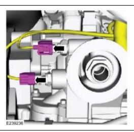
5. Remove the wiring harness bracket nut and position the wiring harness aside.
