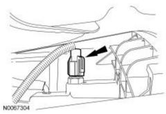
17. Position the transfer case linkage bracket and loosely install the bolt.
