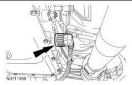
31. Install bolts and tighten to 25 Nm (18 lb-ft).
