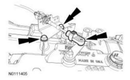
30. Install the transmission vehicle harness connector and lock the transmission vehicle harness connector by rotating the outer shell clockwise.
