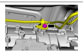
Remove the wiring harness retainer from the transmission and position the wiring harness aside.
