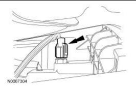
28. For vehicle with electric shift transfer case; disconnect the gearmotor encoder connector and the gearmotor electrical connector.
