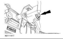
19. Tighten the transfer case linkage bracket bolt to 115 Nm (85 ft-lb).
