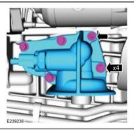
39. Position the wiring harness and install the wiring harness bracket nut. Tighten to 11 Nm (97 in-lb).
