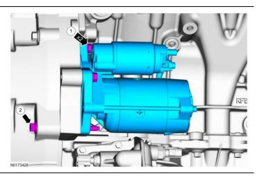
Remove the retainers and remove the starter dust shield.
