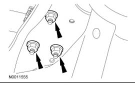
26. Install the 4 RH engine support insulator nuts. Tighten to 115 Nm (85 ft-lb).
