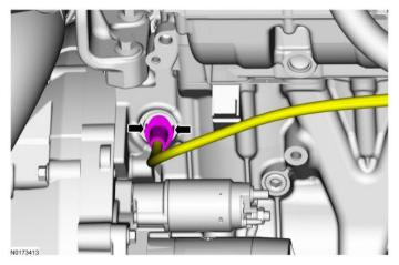
Remove the 3 bolts securing the starter and remove the starter.
