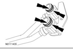
Position the transmission fluid cooler tubes in the transmission case and install the bolt. Tighten to 25 Nm (18 ft-lb).
