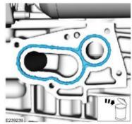
38. Install oil filter adapter and the bolts and stud bolt. Tighten to 12 Nm (106 in-lb)
