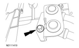
35. Remove the lowers transmission fluid filler tube bolt and position and transmission fluid filler tube aside. Remove and discard the transmission fluid filler tube O-ring.
