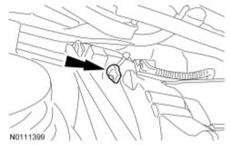
29. Position the selector lever cable bracket and install the 2 bolts. Tighten to 48 Nm (35 ft-lb).
