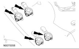
27. For **2017-2019** trucks install the fuel line bracket bolt. Tighten to 85 lb.ft (115 Nm).
