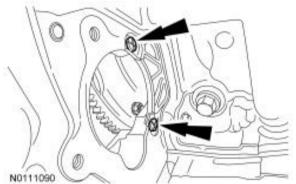
Remove and discard the 6 torque converter nuts.
