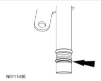
8. Install the transmission fluid filler tube in the transmission and install the lower transmission fluid filler tube bolt. Tighten to 25 Nm (18 ft-lb).
