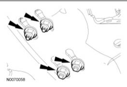
21. Remove the 3 LH engine support insulator nuts.
