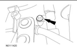
36. Remove the 11 bolts and remove the transmission from the engine dowel pins.
