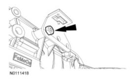
27. Disconnect the 3-position mode switch electrical connector.
