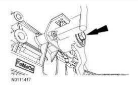
26. Remove the bolt and transfer case linkage bracket.
