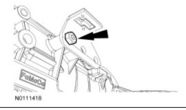
18. Position the transfer case linkage and install the bolt. Tighten to 115 Nm (85 ft-lb).
