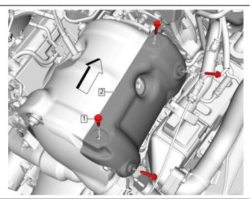
14. Clean and reinstall the exhaust temperature sensor (#2).
