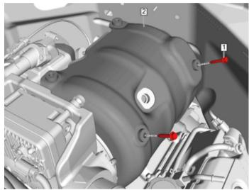
Install the NOX sensor (#1) using a M22 flare nut wrench or socket.
