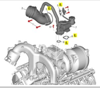
24. Remove the **three** (3) 10mm exhaust gas recirculation valve pipe heat shield bolts (#1) and remove the EGR valve pipe heat shield.
