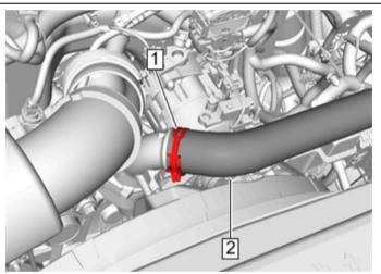
7. Remove charge air cooler band clamp (#1) and remove charge air cooler inlet pipe (#2) from turbo outlet.
