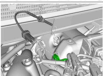
35. Remove the NOX sensor (#1) using a M22 flare nut wrench or socket.
