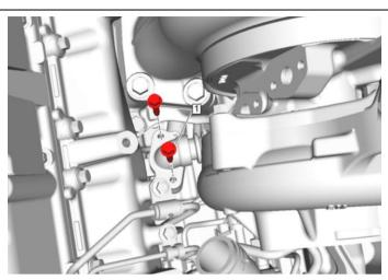
42. Remove the **four (4) 13mm** exhaust front bracket bolts **(#1)** from the back of the catalytic converter and remove the exhaust front bracket **(#2)**.
