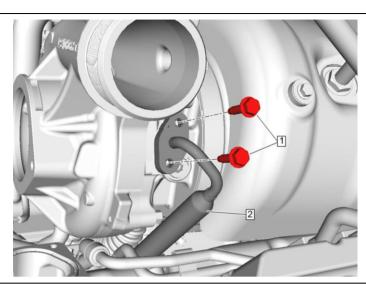
11. Reinstall the left-side turbocharger heat shield (#2) using two (2) 10mm bolts (#1).
