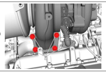
45. Lift the old turbocharger out of the engine.
