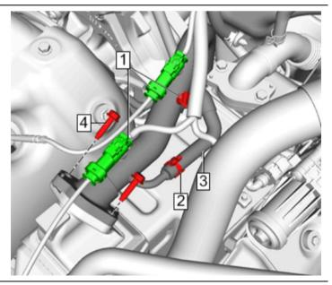
33. Remove the EGR coolant return pipe (#1).
