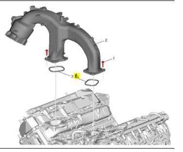
29. Remove the **two (2) 10mm** turbocharger oil feed pipe bolts **(#1)**. Reposition the turbo oil feed line **(#2)** aside.
