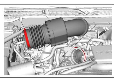
42. Reinstall the air cleaner outlet resonator using **two (2)** band clamps and **one (1) 13mm** nut.
