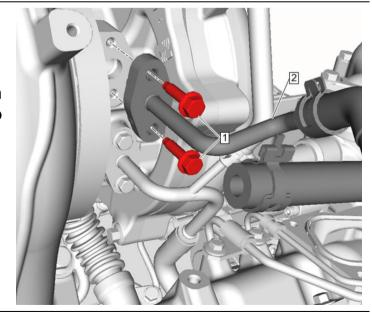
Reinstall turbocharger oil feed pipe (#2) using new gasket and two
