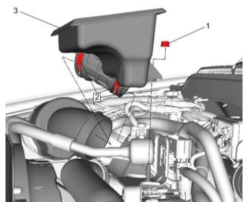
43. Reinstall the CAC inlet pipe (#2) to the turbocharger outlet using an 11mm socket.
