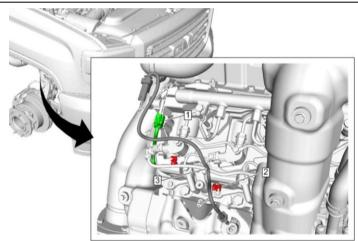
26. Reinstall the EGR pipe heat shield using **three (3) 10mm** bolts.
