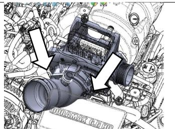
Reinstall the oil filter assembly with the **four (4)** tamper proof screws.
