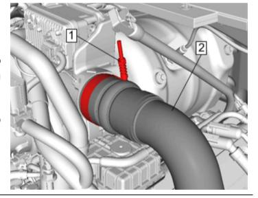
44. Reconnect the vehicle batteries. Refill and bleed the cooling system.
