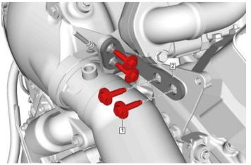
7. Reinstall turbocharger oil return pipe with new gasket and **two (2) 10mm** bolts.
