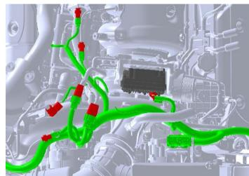
39. Reconnect the alternator electrical connectors.
