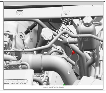
13. Reinstall the right-side turbocharger heat shield (#2) using four (4) 10mm bolts (#1).
