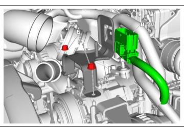
38. Reconnect the engine wiring harness.
