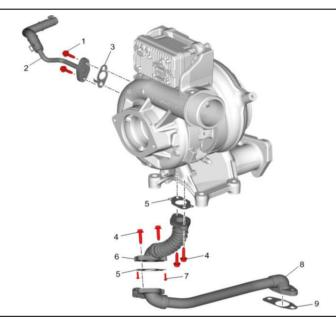
2. Lower the BD turbocharger assembly (#1) into the engine, aligned over the new mounting gasket (#2).
