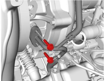
Reinstall turbocharger coolant return line (#2) using new gasket and two (2) 10mm bolts (#1).
