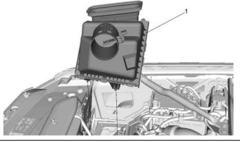
41. Reinstall the air cleaner outlet front duct using **two (2)** band clamps and an **11mm socket**.
