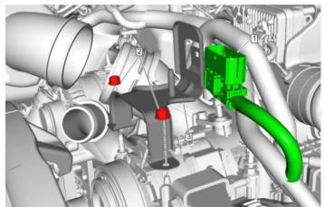
11. Disconnect and reposition the wiring harness as necessary.
