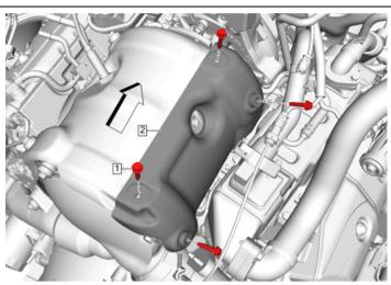
37. Remove the **two (2) 10mm** bolts **(#1)** and remove the left side turbocharger heat shield **(#2)**.
