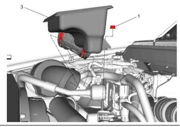
4. Loosen the **two (2)** band clamps **(#1)** and remove the air cleaner outlet front duct **(#2)**.
