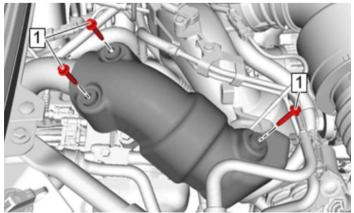
25. Remove the **two (2) 13mm** EGR pipe bolts **(#1)** at the upper intake.
