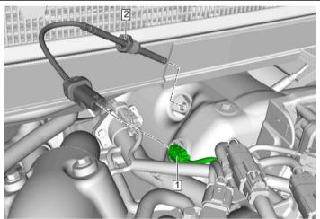
15. Reinstall the EGR coolant return pipe (#1) and align it with the new gasket (#2).
