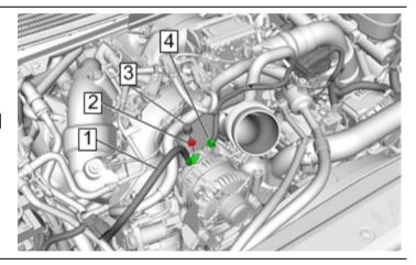
40. Reinstall the air cleaner assembly to its retainers and reconnect the electrical connector.
