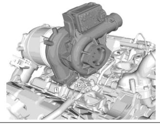
3. Secure the turbine inlet to the exhaust manifold using four (4) 15mm bolts (#1).
