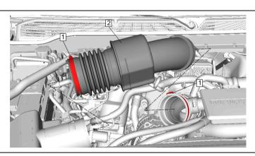
5. Remove the air cleaner assembly from its retainers.
