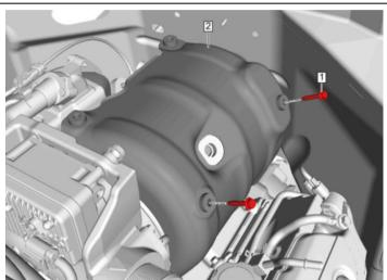
38. Remove the **two (2) 10mm** turbo coolant return pipe bolts **(#1)**.
