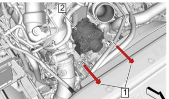
31. Realign the AC compressor and install the **four (4) 15mm** stud bolts.
