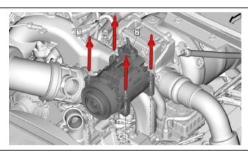
20. Remove the **two (2) 13mm** alternator bolts **(#1)**, then remove the alternator **(#2)**.
