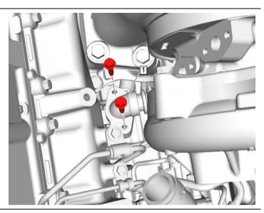
Reinstall turbocharger coolant feed line (#2) using new gasket and two (2) 10mm bolts (#1).
