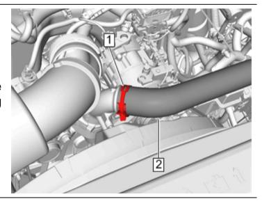
24. Reinstall the EGR pipe using new gaskets and two (2) 13mm bolts (#1).
