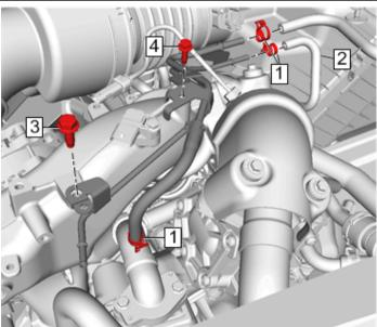
23. Reconnect the radiator inlet hose (#2) to the water outlet with the spring clamp (#1).
