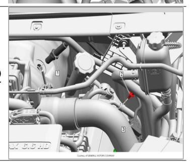
36. Remove the **four (4) 10mm** bolts **(#1)** and remove the right side turbocharger heat shield **(#2)**.
