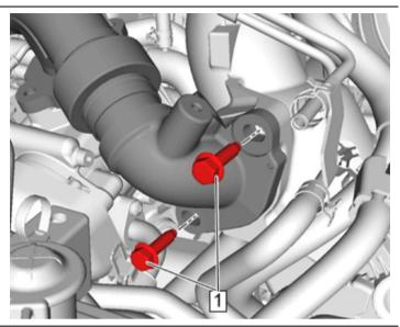
26. Remove the **13mm** (**#3**) and **10mm** (**#4**) bolts from the intake manifold and move the radiator surge tank inlet hose aside.
