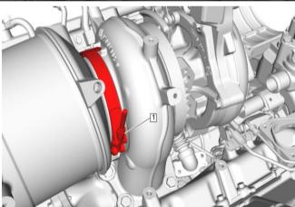
44. Remove the **four (4) 15mm** turbocharger pedestal bolts **(#1)**.
