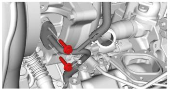
41. Remove the **two (2) 10mm** oil drain pipe bolts **(#1)**.
