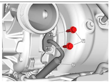
30. Disengage the EGR coolant return pipe hose clamp (#1).
