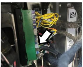
2019: Use a pry tool to release the headlight control cluster to reveal the StarCAN connector as shown.
