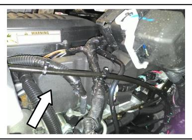
12. Loosen the fittings on the line that goes from the fuel rail to the fuel pump. Once both fittings are loose the line can be removed from the vehicle (19mm).
