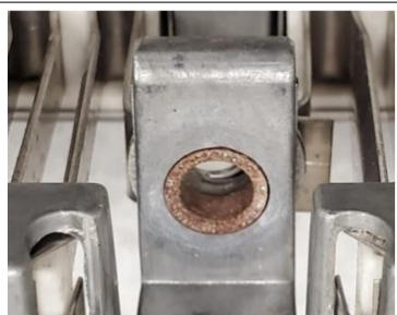
7. Install the new lower busbar between the heater elements using the supplied button head bolt with threadlocker, the new insulating washers and the previously retained steel washer. Hand-tighten for now – this bolt will be torqued at a later step.
