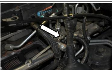
21. Remove the four bolts holding the fuel rail to the grid heater (10mm).
