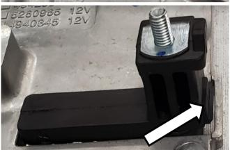
2. To remove the lower busbar, use the included IP25 Torx Plus bit and slim 10mm wrench to remove the bolt and nut in between the heating elements. Retain the steel washer and the small insulating insert that fits in the grid heater mount bolt hole.
