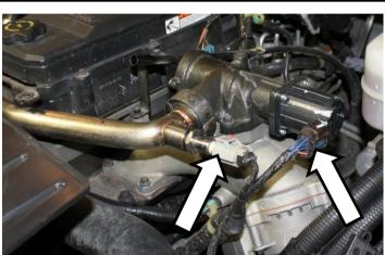
3. Loosen the EGR cross over pipe clamps (11 mm) and slide them down the pipe. Remove the bolt located at the center of the pipe, and remove the pipe from the vehicle (8mm).
