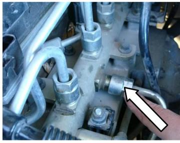
13. Remove the banjo bolt with washer from the front side of the fuel rail (17mm).
