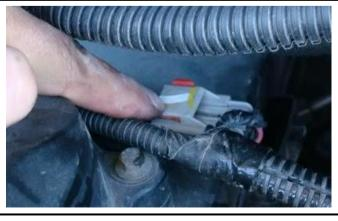
19. Disconnect the EGR servo motor connector.
