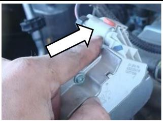
20. Remove the power wire from the grid heater (10 mm).
