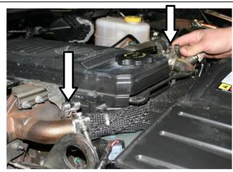
17. Reconnect the EGR valve connector to the EGR valve.
