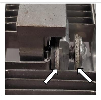
8. Install the new upper busbar assembly into the top of the grid heater.
