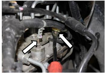
11. Reconnect the throttle valve sensor to the bottom of the intake horn.
