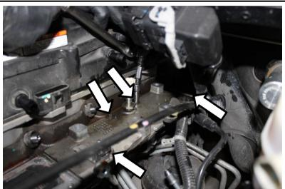
24. With the four bolts removed you may need to gently pry the grid heater from the gasket before it can be removed from the vehicle.
