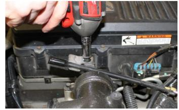
15. Reinstall the harness clip back onto the horn.
