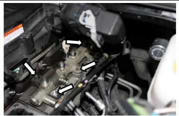
3. Reinstall the six injector lines (19mm), an easy task if previously marked for identification.
