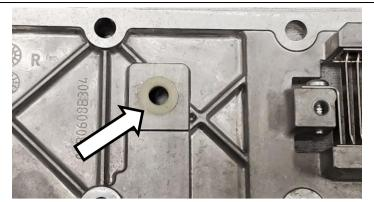
6. Install the small insulating insert into the grid heater mount bolt hole located in between the heating elements.
