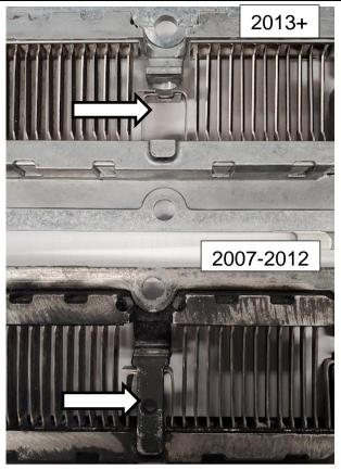
4. For 2007-2012 grid heaters, cut the cast aluminum feature using a rotary tool with cutting disc or hacksaw. Make two cuts flush with the vertical wall in the locations shown on the picture, making sure not to damage the heating elements underneath. The end result after cutting will be a grid heater that looks like the 2013+version as shown above.
