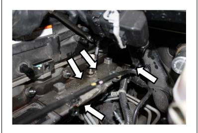
2. Reconnect the fuel rail connector. Then apply some pipe dope to the four OEM fuel rail bolts and install the fuel rail to the intake plate. Torque to 18 ft-lbs (24.4 Nm).
