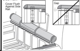
Secure Driver Side Rail to Tonneau Cover Assembly
