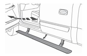
Order to tighten screws: Board to Linkage 1st Linkage to Body 2nd Torque 5-7 ft. lbs. (6.78-9.49 Nm / 60-84 in. lbs.) Do not exceed 7 ft. lbs. of torque
