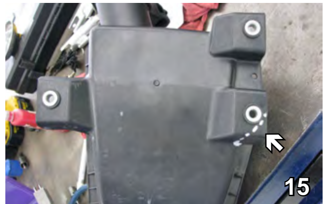
15. On the driver side, trim the corner of the air baffle up to the rubber as shown.
