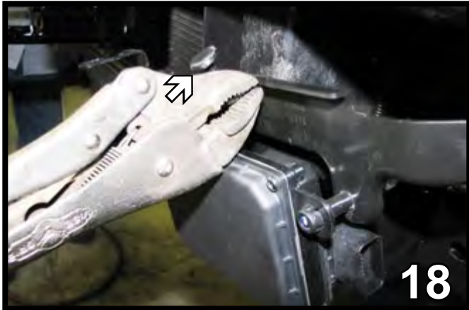
18. If the vehicle has adaptive cruise control, reattach it on the driver's side. Using a vise grip bend the pin downward out of the way.
