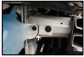
Using a utility knife, remove the outer flange of the washer fluid reservoir as shown.
