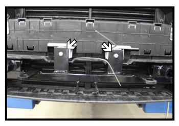
11. Using a 3/8" drill bit, drill the front holes thru the metal brackets. Install 3/8"-16 x 1" bolts, 3/8" lock washers and 3/8"-16 nut plates.
