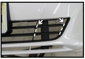
Trim the two (2) horizontal bars from the lower grille opening as shown. Do this on both sides of the fascia. Reinstall the fascia.
