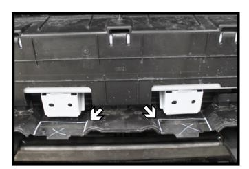
7. Using a utility knife, trim two (2) pockets in the plastic shrouding back flush to the metal brackets as shown.
