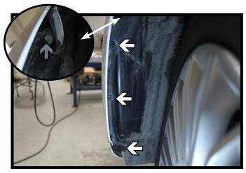
Using a 10MM socket, remove the screw from the top edge of the wheel well (gray). Remove the three (3) push pins from the outer edge of the wheel well (white). Do this on both sides of the vehicle.
