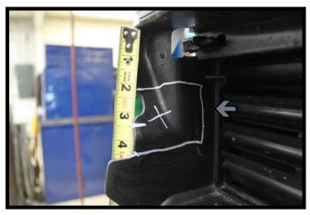
5. Trim the air baffle approximately as shown for baseplate clearance. Do this on both sides of the vehicle.
