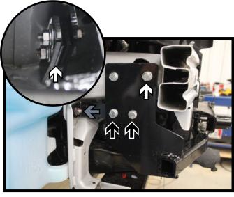
10. Using a 3/8" drill bit, drill the front top hole thru the frame. Install a 3/8"-16 x 1" bolt, 3/8" lock washer and 3/8"-16 nut plate (white). Using a 13MM socket, remove the existing frame nut and install the side bracket with a 8MM flat washer and 8MM nut (gray). Install 3/8"-16 x 1" bolts, 3/8" lock & flat washers and 3/8"-16 nuts into the lower holes (black) with the spacer plate in between the bracket and baseplate (inset). Do this on both sides of the vehicle.
