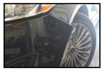
4. Pull the corners of the fascia out and away from the vehicle. Disconnect all electrical connections from the back side of the fascia. Remove the fascia from the vehicle and set aside.
