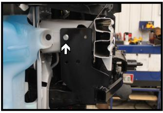
9. Using the existing hole, bolt the baseplate to the frame with a 3/8"-16 x 1" bolt, 3/8" lock washer and 3/8"-16 nut plate. Do this on both sides of the vehicle. Level and tighten down the baseplate.
