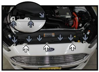
Using a T25 Torx, remove the three (3) screws from the top edge of the fascia (white). Remove the six (6) push pins from the top edge of the fascia.
