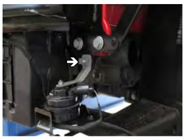
Using a 50 Torx, remove the one (1) screw at the top of the horn bracket, unhook the wiring and set aside. Repeat on other side.
