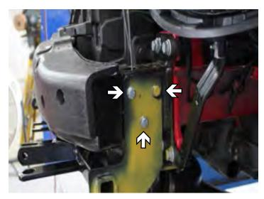
13. Install the three (3) 3/8"-16 x 1-1/4" bolts, 3/8" lock washers and 3/8"-16 nut plates w/wires using the 1-1/4" holes on top of frame to insert nuts. Repeat on other side of vehicle.
