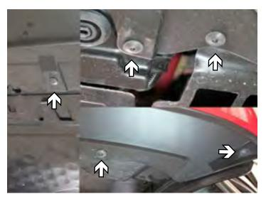
5. Using a 25 Torx remove the ten (10) screws from the underside of the fascia. There are five (5) on each side.
