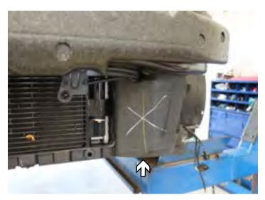
After front fascia is removed, locate and remove the two (2) plastic shrouds at the front of vehicle on both sides. These will not be used during re-installation of front fascia.
