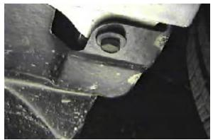
Just forward of front tire on the underside of fascia, remove metric bolt with 10MM socket, both sides. Remove one push pin from opening in fascia. Pull fascia forward and set aside.
