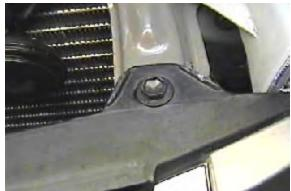
1. Remove the two metric bolts just above head light assemblies with the 10MM socket.
