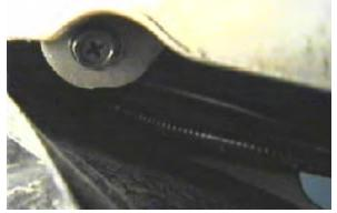
**3.** Using the 10MM socket, remove the metric bolts from fascia corners just forward of front tires and behind wheel well cover, both sides.
