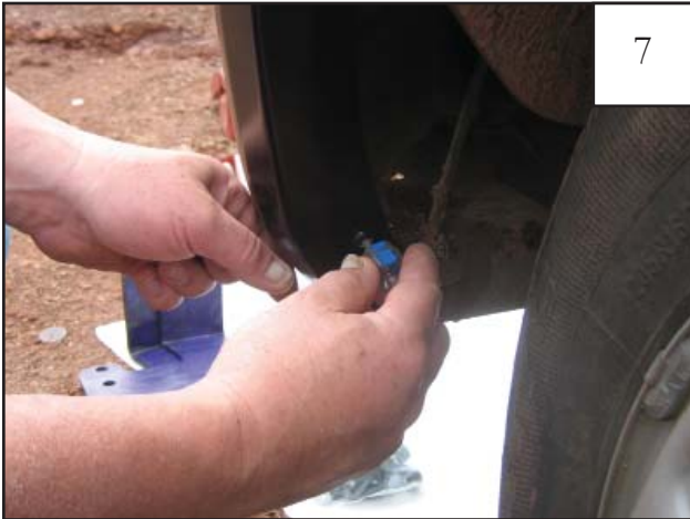
While using a stubby screwdriver, install the supplied Screws (SW1-0050) into the remaining holes in the flare (4 places).
