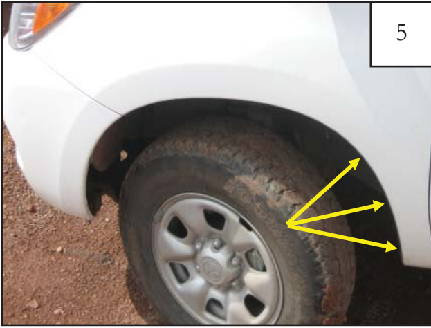
Hole locations for supplied screws (SW1-0036) to be installed in the next step.
