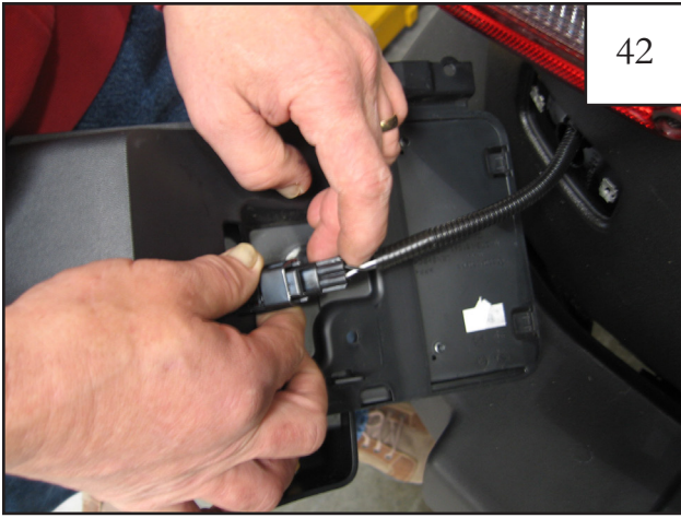
Reconnect light of license plate frame.
