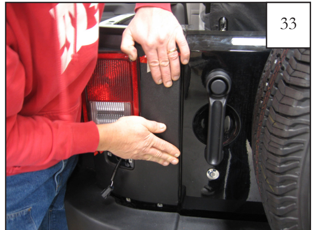
Press firmly on side of part where the two previous tape liners were removed.
