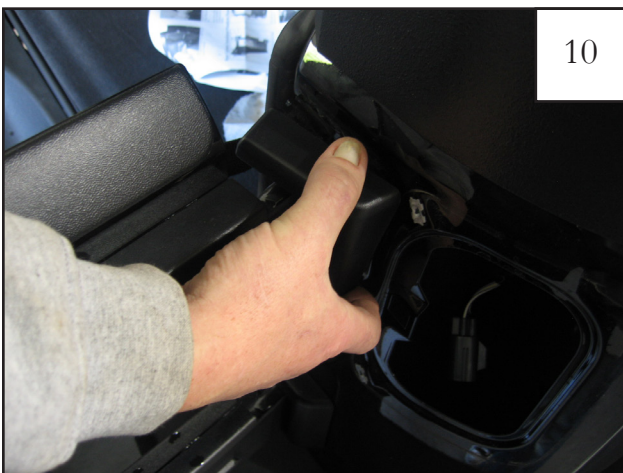
Slide covers off door hinges.
