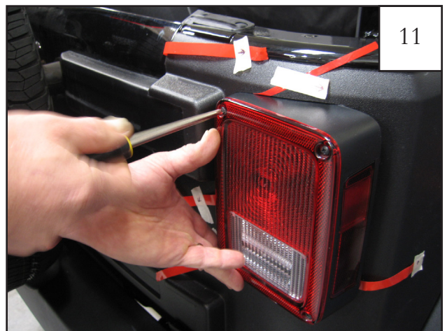
Position part on vehicle and using a #2 Phillips screwdriver, loosely start screws in the two locations they were removed from in the tail light.
