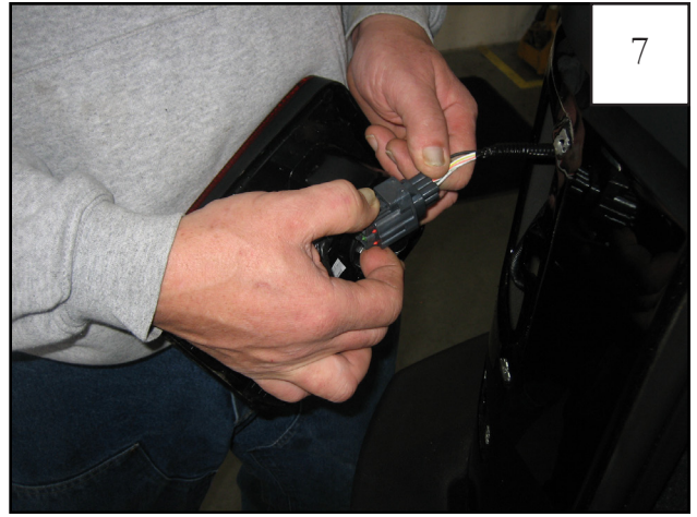
Disconnect the light by pressing down on the connector. Repeat steps 5-7 for passenger side tail light. Clean all dirt and debris from vehicle then use supplied alcohol wipe where part will be. NOTE: Temperature should be at least 60°F for proper tape adhesion.
