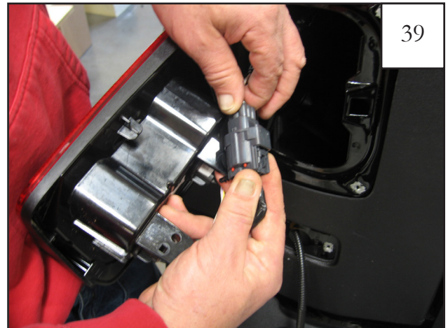
Reconnect light connector of tail light.
