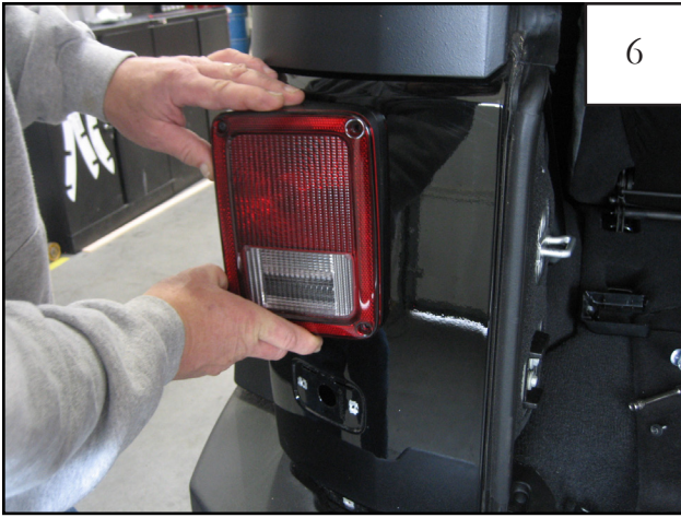
Slide light toward the inside of the vehicle then pull out to remove the tail light.
