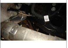
3. Remove the (2) factory M10 hex nuts located behind the license plate. While supporting the bumper, locate and remove the (4) factory M10 hex nuts from the bumper beam. Set bumper aside for reinstallation.
