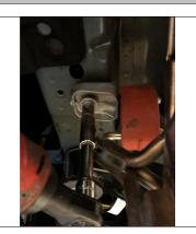
2. Fishwire (2) CM-SP10 spacers and (2) 1/2" carriage bolts through enlarged hole and out mounting holes, both sides. Reverse fishwire (1) CM-SP10 spacer and (1) 1/2" carriage bolt through and out enlarged hole on both sides of vehicle. Use Fishwire and Reverse Fishwire Diagrams as reference.
