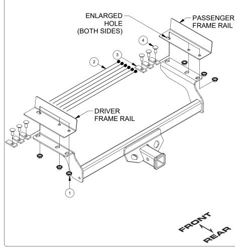
1. Align hitch on vehicle and outline forward most attachment on both sides to use as hole enlargement template. Enlarge forward most hole towards rear of vehicle using marked outline.
