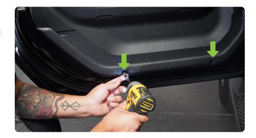
STEP 4 | Slide the DV8 Slim Door Molle Pocket tabs behind the factory door pocket plastic
