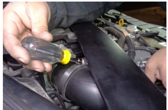
36. Tighten the screw clamps on the coupler. REPEAT ON THE DRIVER SIDE.
