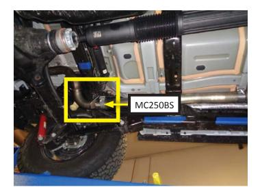
17. Slip a **clamp (MC250BS)** over the muffler inlet of Outlaw muffler. Then slide the muffler inlet over the rear end of rear inlet pipe. Support the muffler, then ensure all connections are completely seated.
