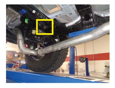
9. Remove bolt on clamp at resonator inlet.
