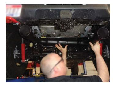
18. Place factory (driver and passenger side) hanger mounts into position, then reinstall and tighten the factory bolts.
