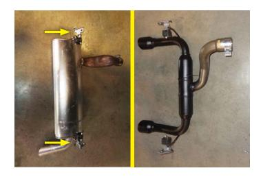
8. Remove stock hanger mount with a pry bar and retain for re-use.
