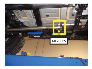
16. Slip a clamp (MC250BS) over the front end of rear inlet pipe (86506S), then slide the pipe onto the rear of the front inlet pipe while pushing the pipe's hanger into the rubber mount on the vehicle. Snug the clamp just enough to allow for adjustment.
