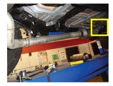
10. Remove resonator assembly from vehicle.
