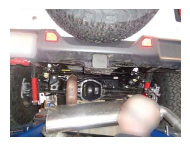
7. Place stock muffler next to Outlaw muffler oriented in the same direction. Then transfer driver and passenger side mounts over to the Outlaw muffler.
