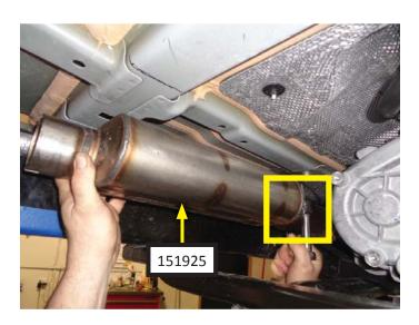
15. Slip a clamp (MC250BS) over the front end of front inlet pipe then slide the front inlet pipe into the back end of the resonator. Make sure the bend on the front inlet pipe is oriented upwards for maximum clearance. Snug the clamp just enough to allow for adjustment.
