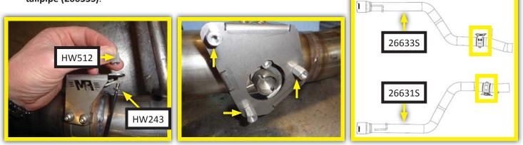
Place driver side actuator onto left tailpipe valve bracket. Place flat washers (HW315) (x3) between actuator and standoff then loosely fasten 3/4" screws (HW240) (x3). Once actuator is located, finish tightening all screws. Repeat step for right tailpipe. (removed step 8)
