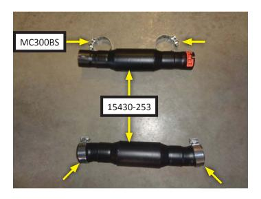
**NOTE:** Mufflers must be installed flat.
