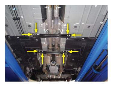
7. Loosen clamps (x2) connecting factory exhaust system to front pipes. Carefully slide system off of front pipes to remove completely from vehicle.
