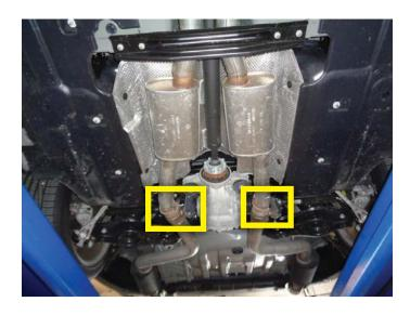
5. Unclip grounding strap and slide wire hanger out of rubber isolator on driver side tailpipe. Next, unbolt mount, flip it around and reinstall. Repeat step for passenger side tailpipe.
