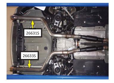
18. Fasten factory bolt and mount into position to secure left tailpipe. Repeat step for right tailpipe
