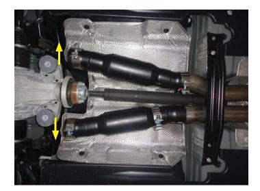
17. Place left tailpipe into muffler while seating wire hanger in rubber isolator. Plug wire into exhaust valve actuator and clip in grounding wire. Repeat step for right tailpipe.
