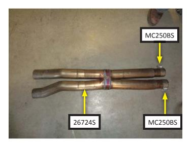
Slide scavenger pipe into front pipes then tighten both clamps just enough to allow for adjustment. Tighten nuts (x8) to install braces which support scavenger pipes. (removed step 6)
