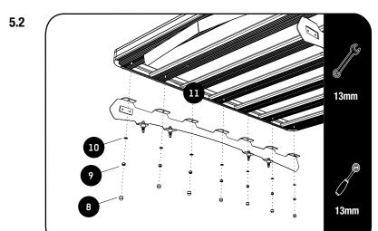
Fit your roof rack to the Foot Rails using M8 x 20 Hex Bolts, M8 x 16 x 1.6SS Flat Washers and M8 Nyloc Nuts (Items 9, 10 & 11).
