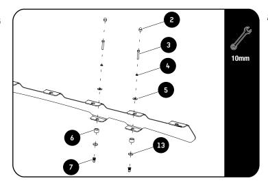
Place a bead of silicone onto the thread of each Hex Bolt before fastening.
