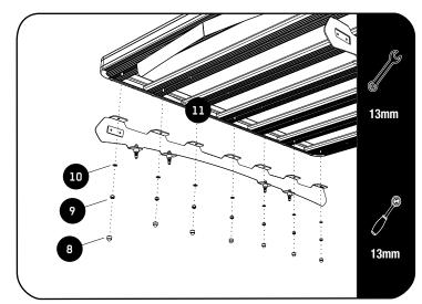
Fit your roof rack to the Foot Rails using M8 x 20 Hex Bolts, M8 x 16 x 1.6SS Flat Washers and M8 Nyloc Nuts (Items 9, 10 & 11).
