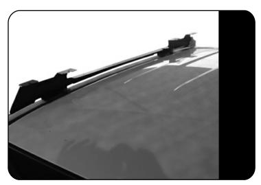
Place the various sections of ditch moulding back into position on the vehicle's roof.
