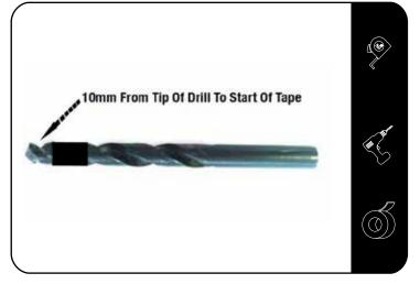
before drilling the holes in the roof, take both 5 & 12 mm drill bits and wrap a band of insulation tape around the drill bits to act as a stopper to prevent you from drilling to deep as there are airbags located below where you will be drilling.
