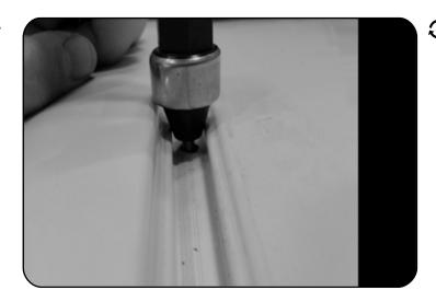
Using a Rivnut Tool, insert an M6 Rivnut (Item 7) into each of the eight 9mm holes drilled in Step 4.3.
