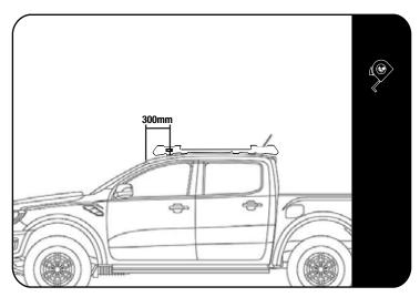
Starting at the top edge of the vehicle's windscreen, measure and mark the dimension as shown onto both LH / RH ditch centre's.
