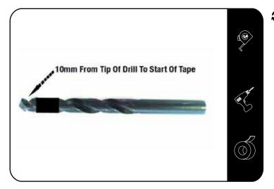
Before drilling the holes in the roof, take both 4 & 9 mm drill bits and wrap a band of insulation tape around the drill bits to act as a stopper to prevent you from drilling to deep as there are airbags located below where you will be drilling.
