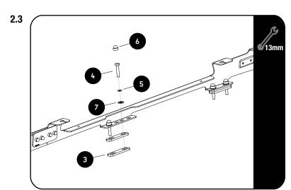
Secure the Foot Rails to the vehicle using M8 x 40 Hex Head Bolts, M8 Spring Washers, M8 x 19 x 2 Flat Washers and Plastic Spacers (Items 3, 4, 5 & 7) as shown.
