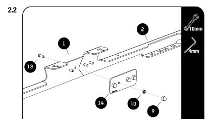
Assemble the Front and Rear Foot Rails (Items 1 & 2) using the Joiner Plate (Item 14) and M6 x 12 Button Head Bolts and M6 Nyloc Nuts (Items 10 & 13) as shown.
