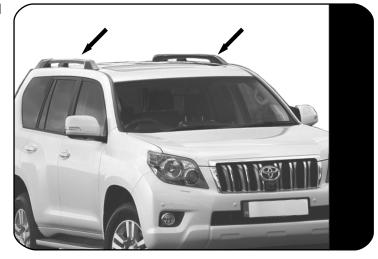
$\ensuremath{\mathcal{L}}\xspace$  Remove the OEM rails from the left and right side of the vehicle.
