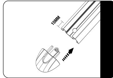
Should you wish to fit the End Caps to the Rail, you will need to drill a 8.5 mm Hole 15mm in from each end as shown. Only fit the End Caps once the Tie Down Rail has been fitted to the vehicle and the Channel Nut has been inserted. (Refer to Step C).
