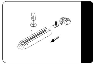
Once the Rail has been secured in position, slide the T-Bolt into the Tie Down Rail. Fasten the Eye Nut and shown.
