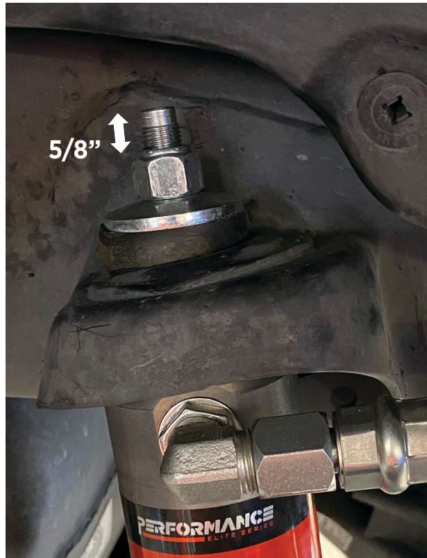
Fig 3: Tighten till there is 5/8" visible stem length.
