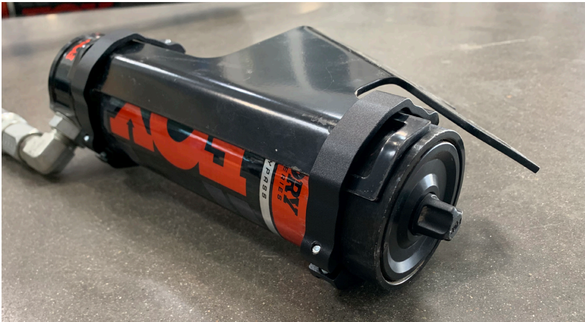
Figure 8: This image is for informational purposes only to demonstrate how the reservoir brackets should interface with the bracket. Mount Group A and B brackets to the vehicle before you install the reservoir.
