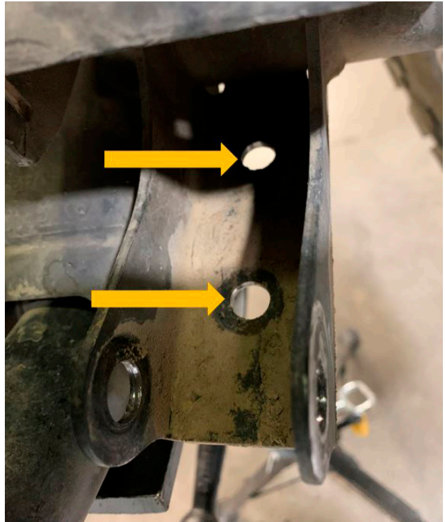
Figure 2: Open up two holes on the bottom of the factory shock mount.
