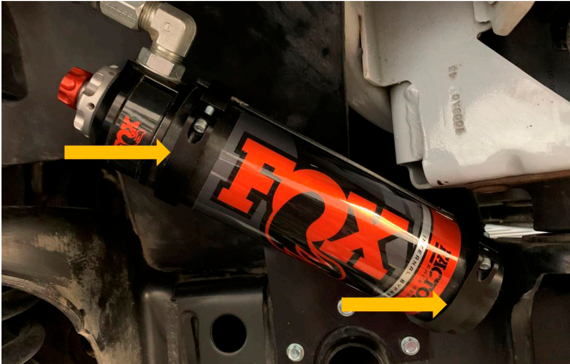
Figure 7: The Group D clamps secure reservoir to Group A and B brackets.
