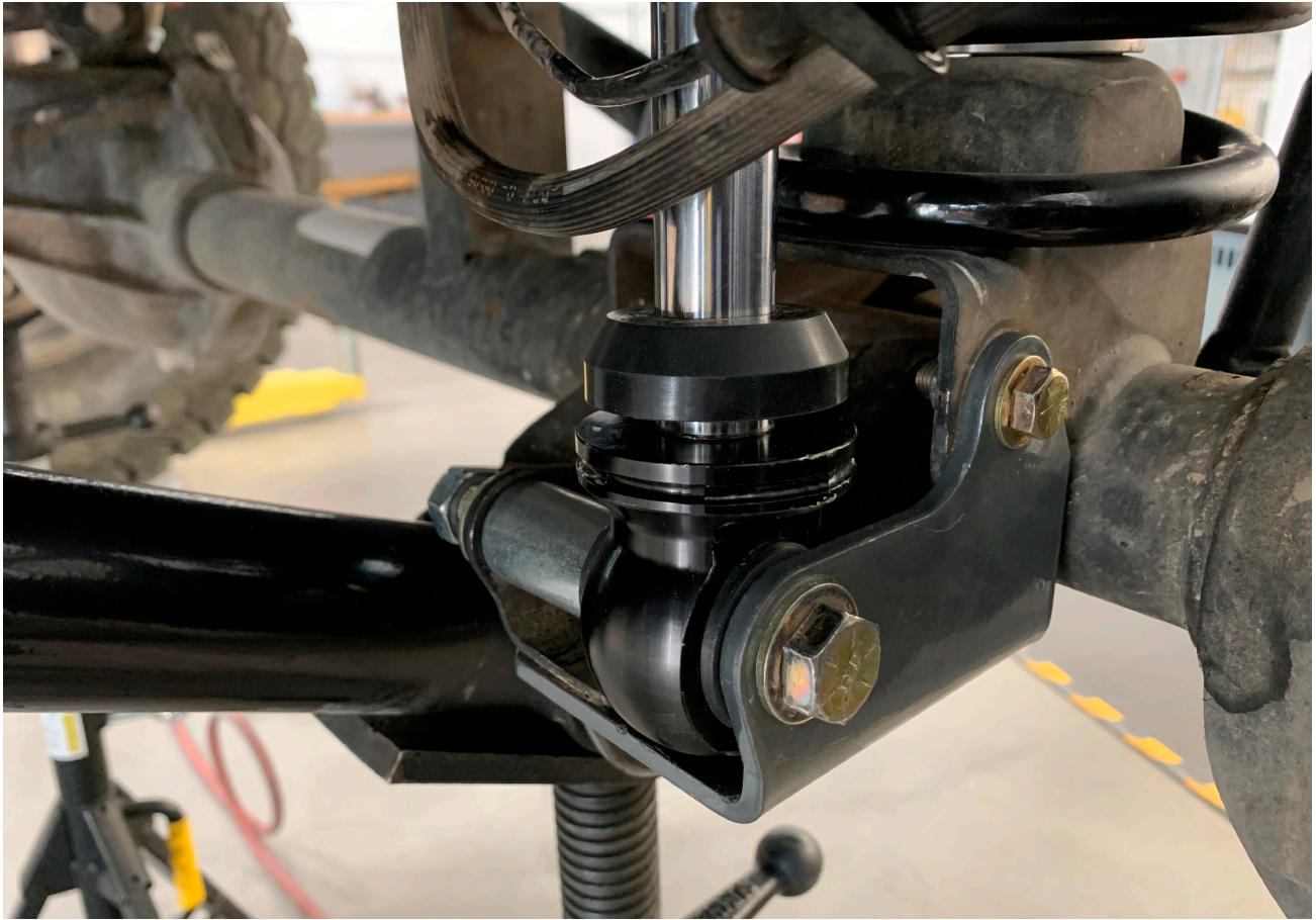
Figure 6: Torque shock hardware to factory specifications.
