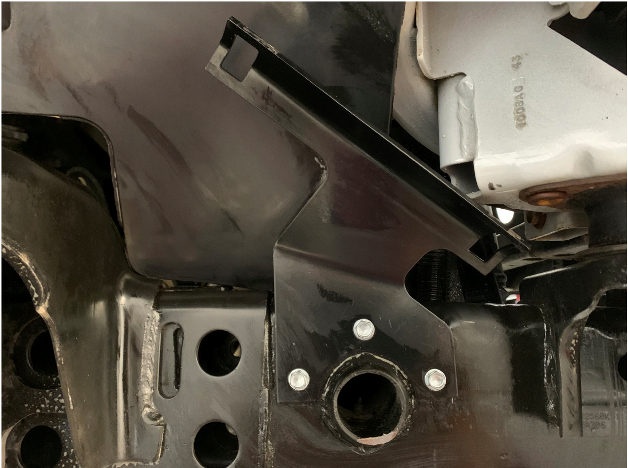
Figure 1: Install the supplied reservoir brackets, Group A and Group B.
