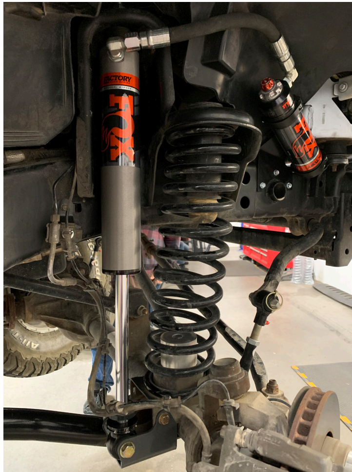
Figure 5: Hand tighten all hardware first.
