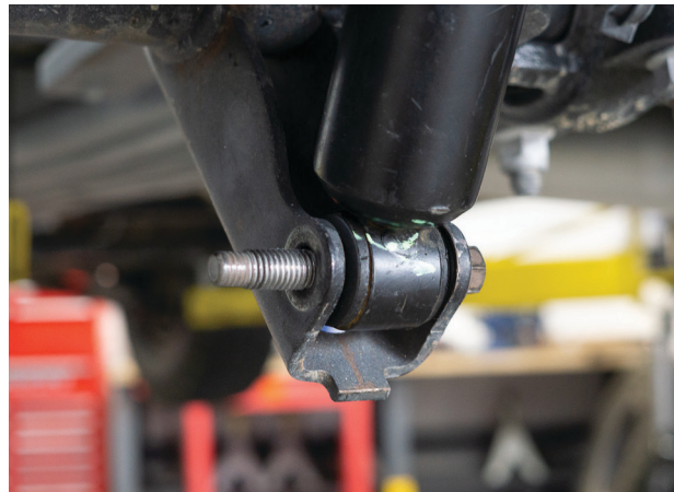
Fig. 20: Remove lower shock mount bolt.
