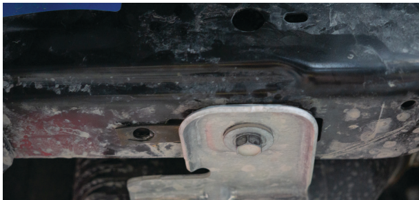
Fig. 8: Use a speed nut in front of the bracket.
