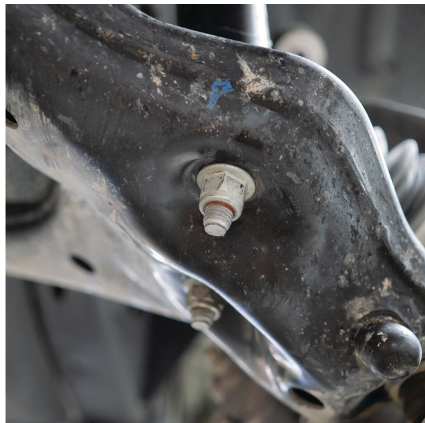
Fig. 7: Remove the bar-pin nuts.
