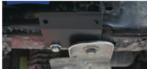
Fig. 9: Install the reservoir bracket.
