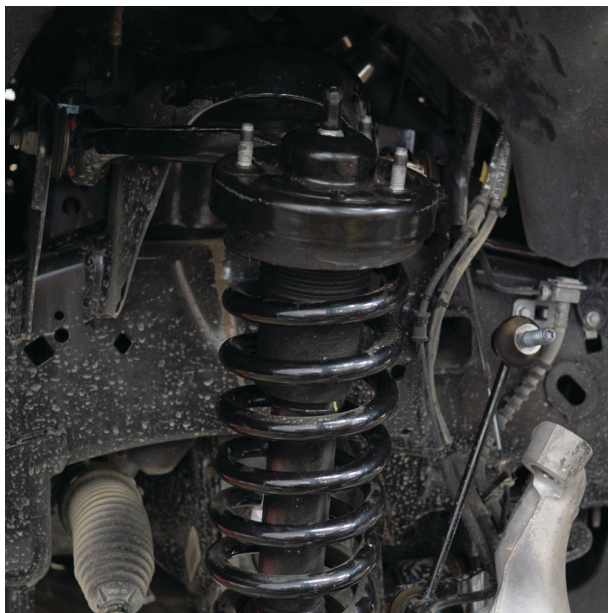
Fig. 6: Free the coil-over.
