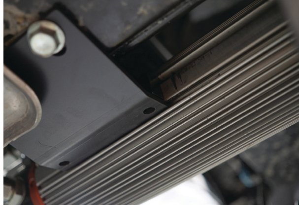
Fig. 11b: Reservoir interfaced with the bracket.
