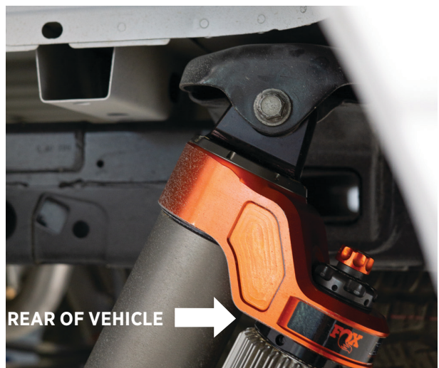
Fig. 21: Install the upper shock mount.
