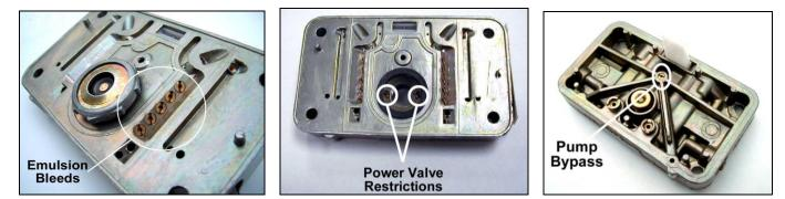
NOTE: The emulsion bleed tuning kit (P/N 36-322) is designed to support the tuning efforts of this new block. It contains ten each of the following bleed sizes: Blank (no hole), .020", .031", .040", .046", and .052". Individual bleeds are available from blanks to .078" from your Holley dealer under individual P/Ns 142-xx (xx=size).
