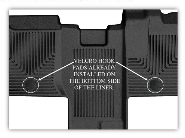
ENSURE THE FLOOR IS CLEAR OF ALL DIRT AND DEBRIS BEFORE INSTALLING THE LINER. THE LINER COMES WITH 2 SETS OF ADHESIVE BACKED VELCRO PADS TO HELP SECURE THE LINER TO THE FLOOR.
