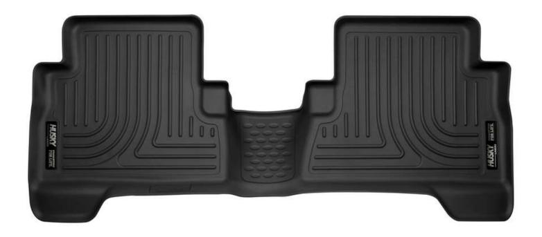
TO EASE THE INSTALLATION OF YOUR REAR FLOOR LINER, FIRST MOVE BOTH FRONT SEATS COMPLETELY FORWARD. THEN, INSTALL YOUR LINER ORIENTED AS SHOWN ABOVE. ONCE YOU HAVE INSTALLED YOUR LINER, REPOSITION THE FRONT SEATS AS DESIRED.
