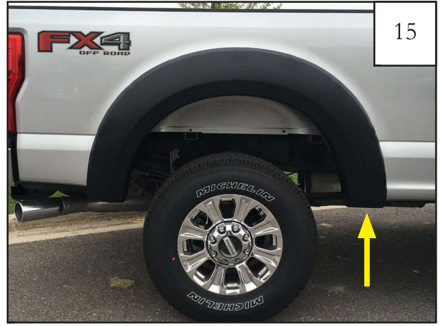
15 Start a supplied screw (SW1-0050) through the flare into the clip installed in Step 13. Tighten all screws.
