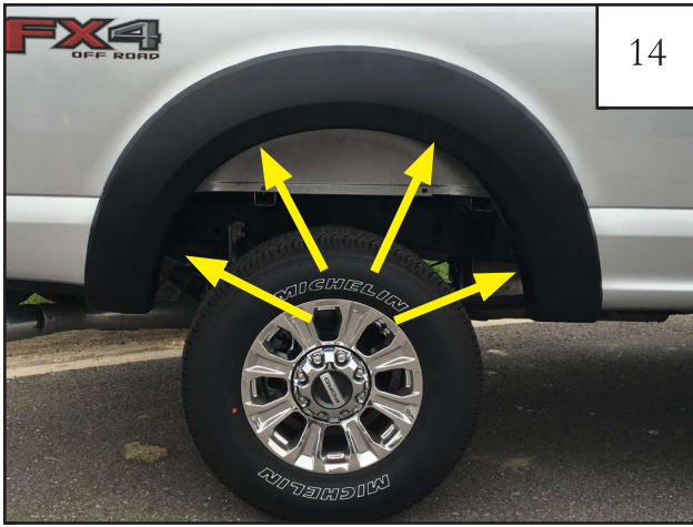
14 While holding flare to vehicle, start supplied screws (SW1-0058) through the four topmost mounting holes in flare and into the clips installed in Step 12.
