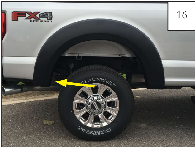
16 Install supplied push retainer (RV1-P0001) into flare and through factory hole at rear of wheel well.
