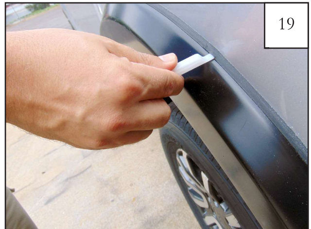
19 Using flat end of supplied Edge Trim Tool (ET1-0002), seat edge trim against flare by inserting straight end between edge trim and flare at one end. Next, slide around entire edge to the other end.
