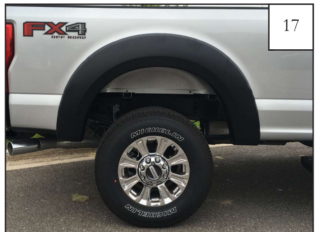
17 Completed rear flare installation.
