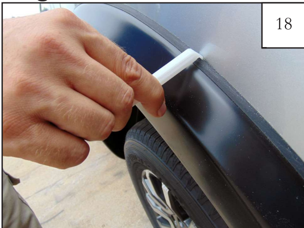
18 Using supplied Edge Trim Tool (ET1-0002), seat edge trim against vehicle by hooking curved end under edge trim at one end of flare. Next, slide around outer edge of flare to the other end.
