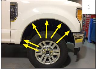
Remove six factory screws with a 7mm socket wrench. Save screws for reinstallation.
