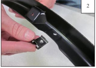
Verify 3 "U"clips installed on the inner bracket as shown. If they are not installed, attach 3 "U"clips (CL1-0022) to the inner bracket as shown.
