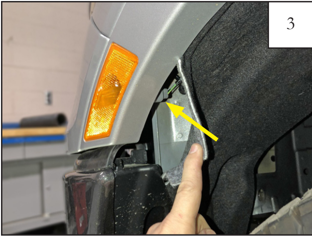
Pull back the fender liner near the front of the fender and locate the side marker light assembly and wiring.
