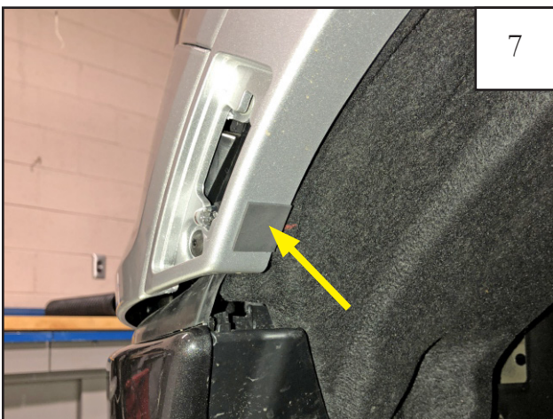
Install (1) black mylar tab (MT1-0014) around the edge of the fender trim aligned with the grease pencil marking.
