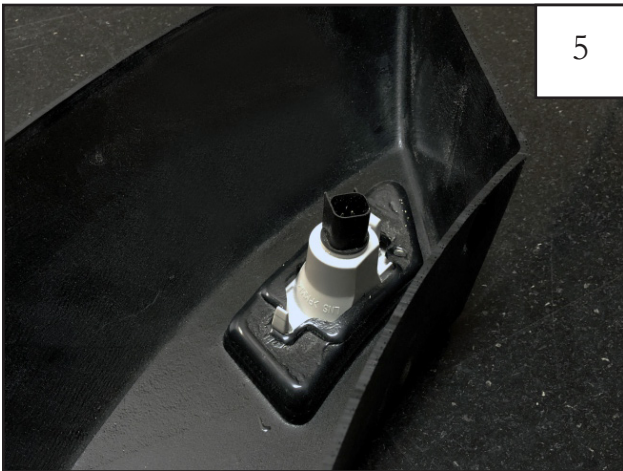
Install the side marker light assembly into the front driver side flare.
