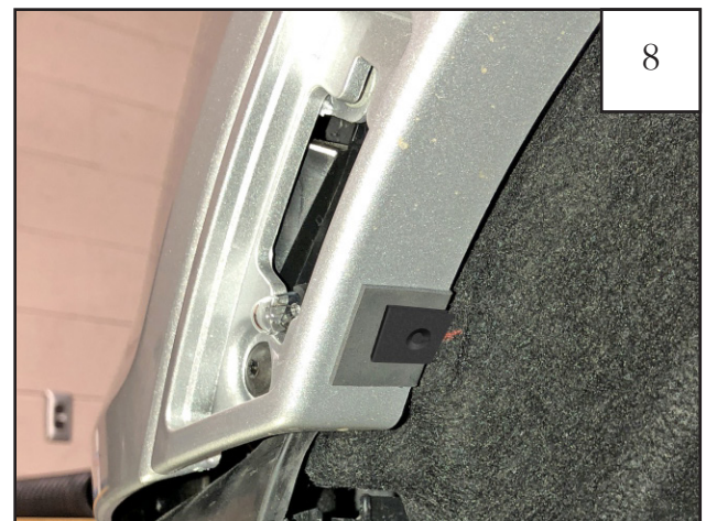
Install (1) "S" spring clip (CL1-0005) over the black mylar tab, centered with the grease pencil marking.
