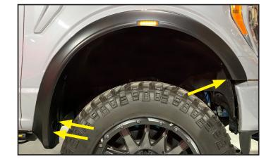
Hold flare to fender, re-install three factory screws removed in Step 6 using sockets and wrench.
