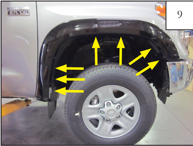
Ensure flare is properly positioned and tighten all screws. Installation Complete. (See steps 5-7)
