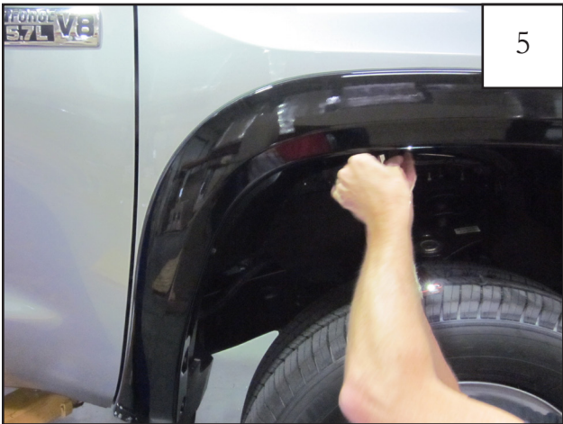
Place flare on fender, aligning holes with clips on the bracket. Start two supplied 20mm Hex Screws (SW1-0036) through two holes on the top of the flare and into clips.
