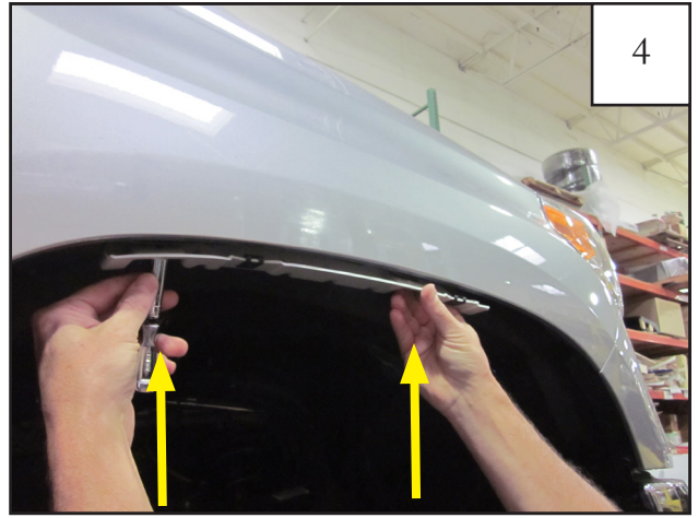
Using two supplied 20mm Hex Screws (SW1-0036), attach bracket to factory holes with a 10mm socket.
