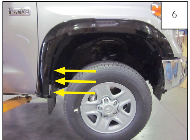
Start three supplied 20mm Hex Screws (SW1-0036) through three rear holes in flare and into factory holes in rear of wheel well.
