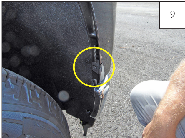
9 Install supplied Tab (MT1-0017) over the front location marked in Step 6. Install a clip assembly as indicated, on top of the Tab. See Step 10 for detail of clip attachment.
