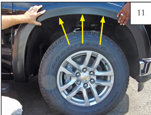
11 Hold flare to vehicle and re-install (3) factory screws (removed in Step 4) with a T15 bit. Do not tighten.
