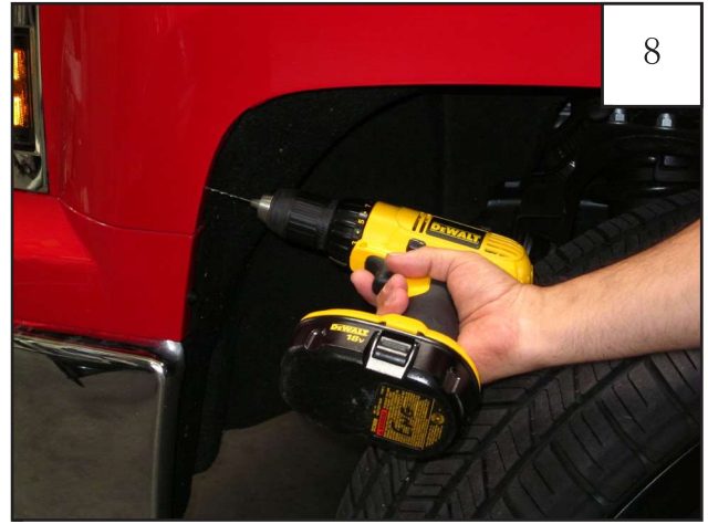
Using a 3/32" drill bit, drill pilot holes at the marks made in Step 7.
