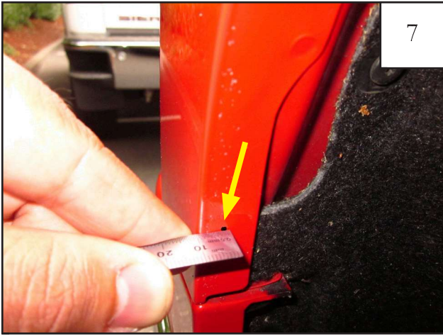
Remove the flare. At the marked location made in Step 5, measure inward 10mm from the edge of the fender. These are the marks to be drilled. Note: Marks at 10mm may be on either side of the first mark.
