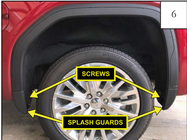
Remove the rear splash guards using a T-15 Torx driver and retain (2) outboard screws for later use.
