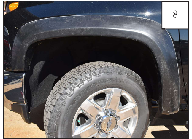
Completed front flare installation. Repeat procedure for opposite side.
