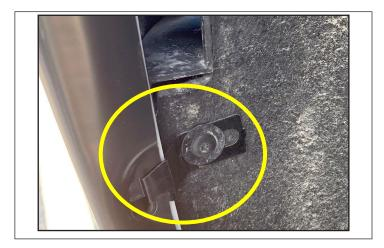
Press flare firmly against body and tighten all screws.
