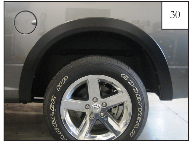
Completed rear flare installation.
