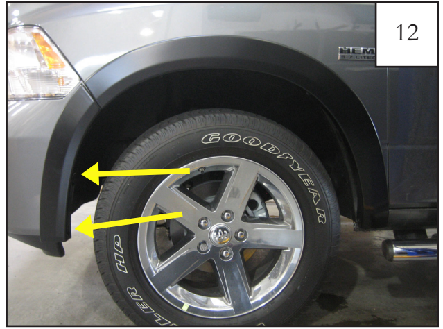
PLASTIC BUMPER ONLY: Additional supplied screw locations.
