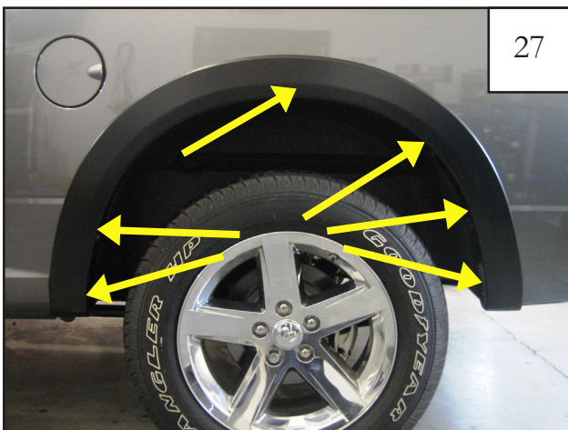
Supplied screw locations. Install one supplied screw at the top of flare first for easier installation. See step 28.
