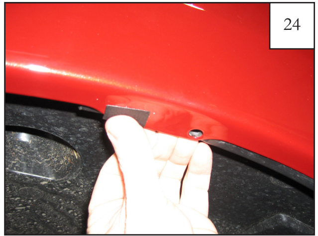
Install plastic tab over existing factory hole.
