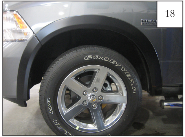
PLASTIC BUMPER ONLY: Completed front flare installation.
