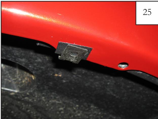
Install speed clip over plastic tab.
