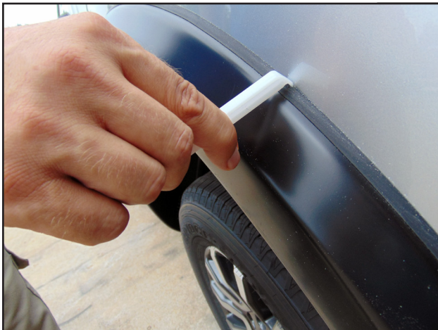
Using supplied Edge Trim Tool, seat Wiper Style Edge Trim against vehicle by hooking curved end under edge trim at one end of flare. Next, slide around outer edge of flare to the other end.
