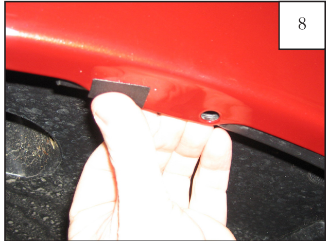
Install two tabs (MT1-0002) over factory holes. There are two factory holes near the rearward arrow. The correct hole for install is the one more toward the front of the vehicle.
