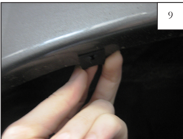
Install #10 U-Clip (CL1-0022) over tabs and existing factory holes. See step 7.
