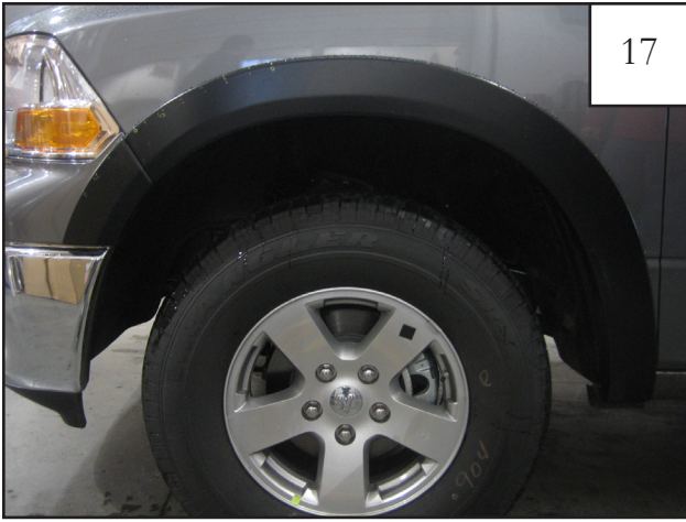
METAL BUMPER ONLY: Completed front flare installation.
