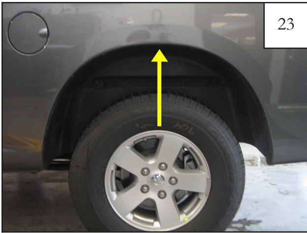
Install #10 U-Clip in this location. See step 25.
