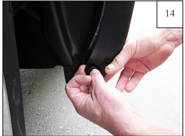
2011 Models Only (Ignore Spacer for other model years, just install screw): For rearmost lower factory screw location, slide factory screw through hole in flare, install supplied 1/2"x.257"x1/2" Nylon Spacer over factory screw, and start factory screw with an 8 mm socket wrench. Do not tighten.
