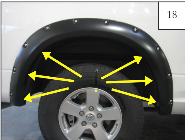
Hold flare to vehicle and start re-installing the (6) factory screws with a 8mm socket. (Part number 50937 uses (5) screws only.) Do not tighten.
