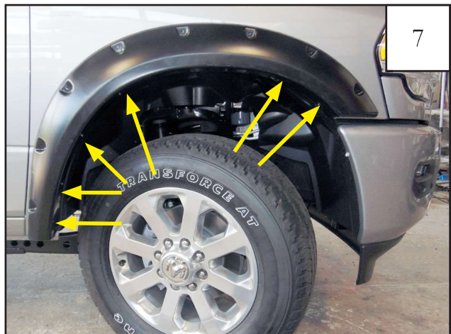
Hold flare to vehicle and start re-installing the (6) factory screws with a 8mm socket. Do not tighten.
