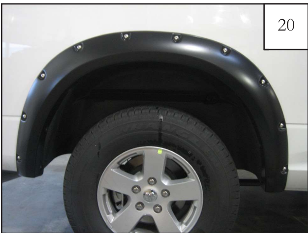
Completed rear flare installation.
