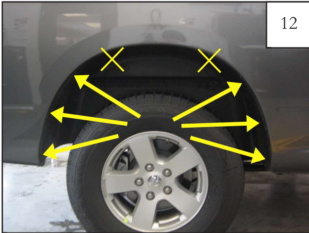
Remove these (6) factory installed screws using an 8mm socket wrench. X's indicate a factory screw that will not be removed. Retain screws to be re-used to install the rear flare. (Part number 50937 uses (5) screws only.)
