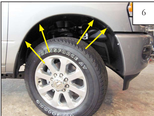
Remove and keep (4) factory installed screws. The screws will be re-used to install the front flare.
