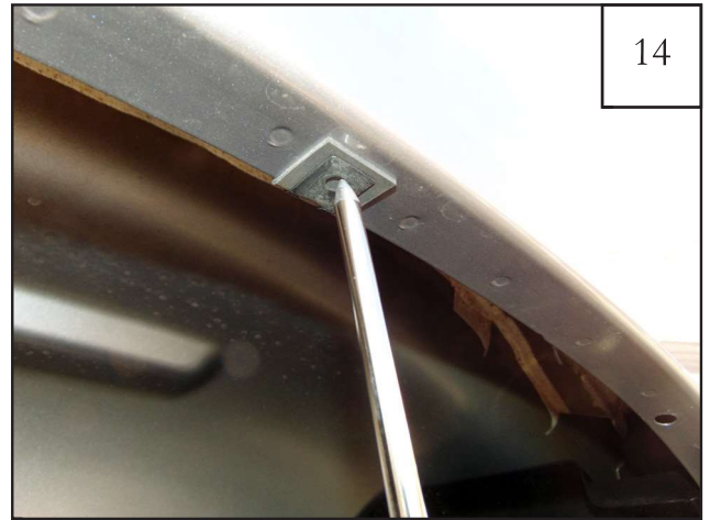
Using an awl or similar pointed tool, poke a hole through Tab (MT1-0014) using the Clip (CL1-0022) hole as a guide. Repeat Steps 12-14 for remaining (2) empty hole locations.
