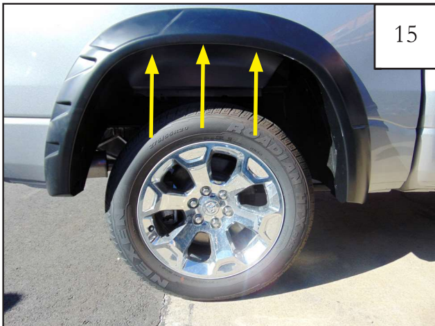
Hold flare in place and start Screw (SW1-0056) using a Phillips screwdriver in (3) locations as shown. Do not tighten. Continue to Step 18.
