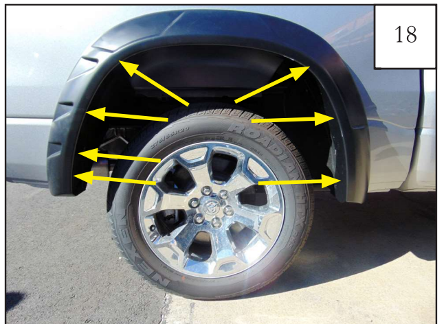
Continue holding flare in place while you start re-installing (7) factory screws using an 8 mm socket wrench. Do not tighten.
