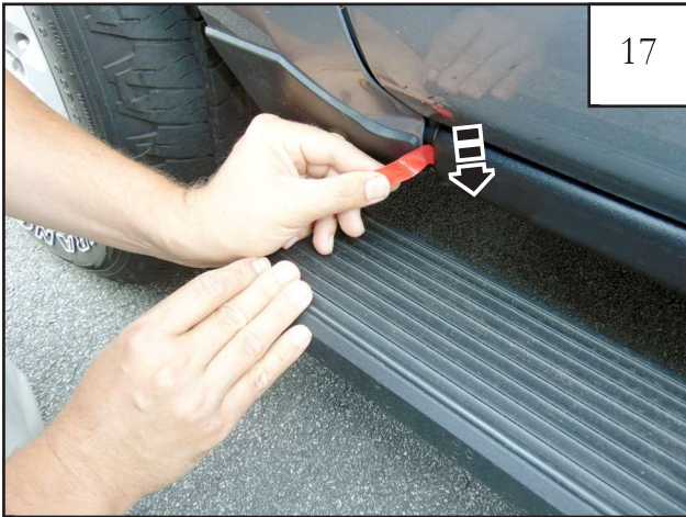
Pull tape liner tab 5. NOTE: It may be necessary to partially close door in order to access tab.
