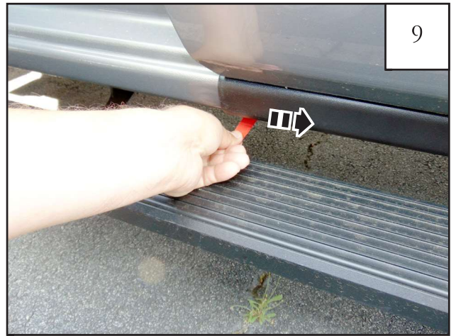
Pull tape liner tab 6. NOTE: It may be necessary to partially close door in order to access tab.
