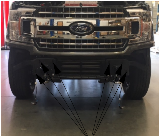
Step 2. Remove lower bumper retaining bolts
