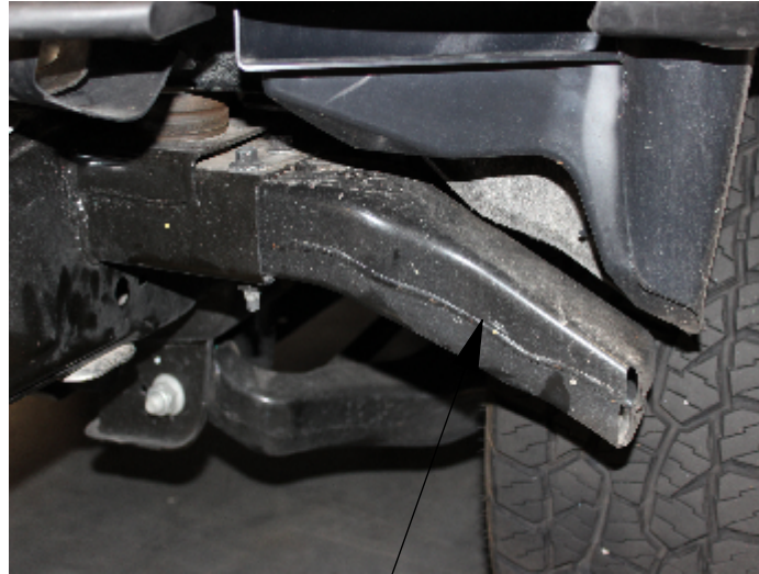
Step 3. Cut/Remove Inner Fender Crash Bars If So Desired.
