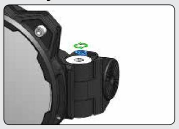
Loosen the M4 Socket-cap Adjustment Screws from End Mounts on both sides of the bar to allow alignment and self-centering.
