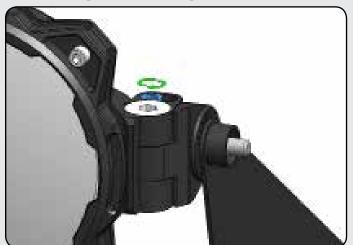
Set the final level and pitch of the Pro6: 1) Tighten the M8 Horizontal Mounting Hardware, allowing the Pro6 to center itself. Then, 2) Tighten the M4 Adjustment Screws to lock Pro6 into position.
